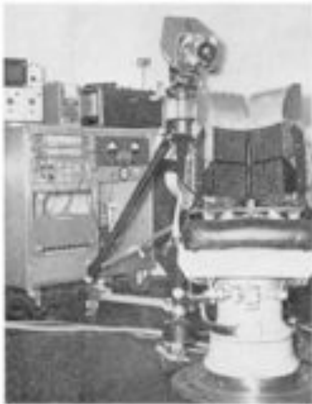
Figure 1: The experimental set up used by Bachy-Rita and his colleagues in their original TVSS experiment [9]. The subjects sit in the chair and their backs are stimulated by four hundred solenoids whose activity is driven by the camera. Subjects can move the camera and also adjust its focus, thereby changing the tactile stimulation on their backs. Over time, blind subjects learn to recognise objects.
