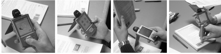
Fig. 1. Usability test tasks: (L-R) button press, icon size, Socket scanning, and Baracoda scanning
