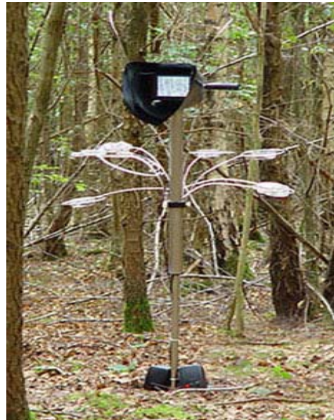
Figure 3: Periscope with screen and RF-tagged plates for triggering information displays
