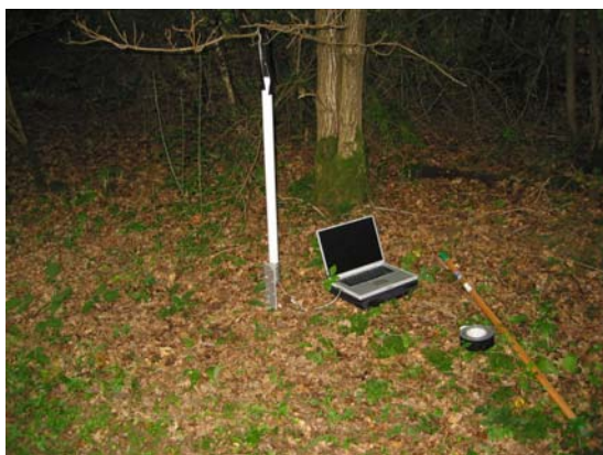
Figure 4: Booster antenna for 802.11b network
