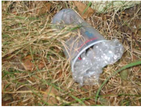
Figure 9: Pingers protected in a plastic cup
