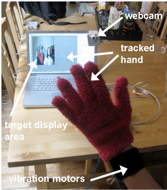
Figure 4. The experimental set up for testing whether two vibration motors could guide arm movements in one and two dimensions. The subject wears a coloured glove on their moving hand that is tracked using a webcam and computer vision software. Subjects position their hand at a central starting point on the display area and then have to move their hand as quickly as possible to a target location. In some conditions the target position is shown with a brief visual cue. Vibrotactile feedback from two vibration motors provides information about the hand's proximity to the target in some of the test conditions.
