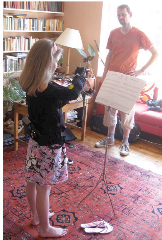
Figure 1. Tracking the bowing action of a young violin player who is wearing the Animazoo IGS-90-M motion tracking system. The movement of her bowing arm and the position of the violin are tracked using 6 inertial measurement units. The motion capture data are transmitted wirelessly to a laptop.
