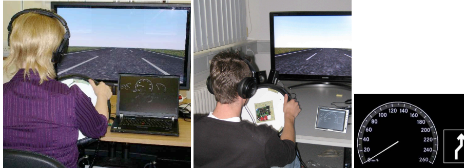
Figure 2. Setup in the first study with the control panel on a laptop (left), setup in the second study with control panel on a 8'' display (middle) and a close-up of the control panel with an direction arrow used in the second study (right).
