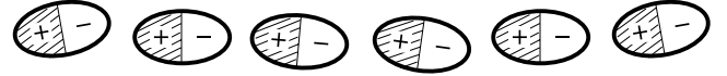
FIG. 2.— Schematic illustration of a chain of dust grains. Dust grains in a low-gravity environment have been found to form aggregates with a low fractal dimension. This may be due to particles having an electric dipole, causing them to form chains. (In this schematic illustration we show a perfect dipolar chain, which would lead to a fractal dimension of unity; in reality there are numerous reasons why the chain can be branched.)
