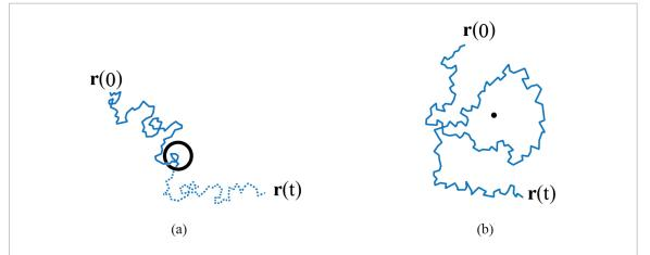
**Figure 2.** Diffusion is a consequence of molecules following a random walk trajectory. Some of these trajectories allow crossing of the ER sheets. In the case of a 'window', the trajectory has to make contact with the singularity (a), whereas in the case of a spiral dislocation, the trajectory only needs to wind around the singularity (b).
