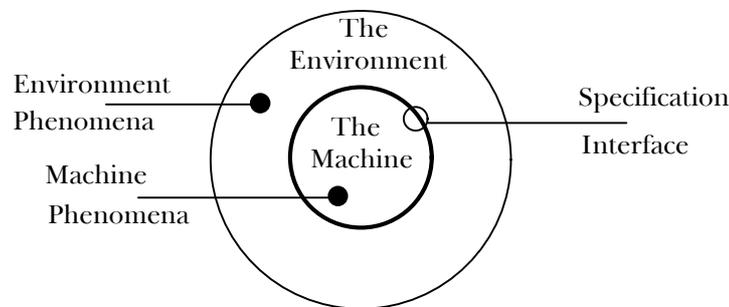
Problems and requirements are to be expressed solely in terms of the environment phenomena. Programs are to be expressed solely in terms of the machine phenomena. The bridge between them is formed by specifications, which are expressed in terms of the phenomena common to the environment and the machine.
