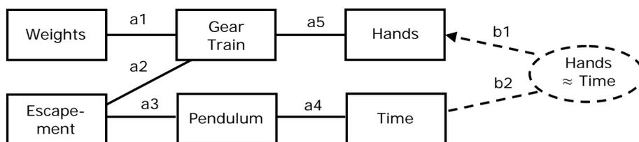
Figure 1. A Pendulum Clock and its Purpose
