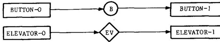
BUTTON-0 is the real button in the real world; it is connected by data stream connection to BUTTON-1, which is the process in the system which models its behaviour. There are sixteen instances of BUTTON-0 and hence of BUTTON-1: 6 within the elevator itself, 5 “up” buttons at floors 1 to 5, and 5 “down” buttons at floors 2 to 6.
