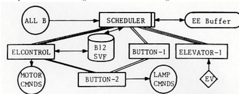
The state vectors of the BUTTON-1 and BUTTON-2 processes have been separated from the executable text, and have been combined into one state vector for each pair, stored in a directly accessible store B12SVF. BUTTON-1 is inverted with respect to its input stream B, and BUTTON-2 with respect to its merged input stream EB&BB.
