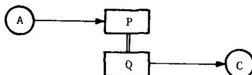
The “write B” operations in P are implemented as calls to Q. it is possible to implement systems of several processes in this way. A sufficient condition for such an implementation is: the system forms an acyclic undirected graph when each process is regarded as a node and each data stream connecting two processes is regarded as an arc.
