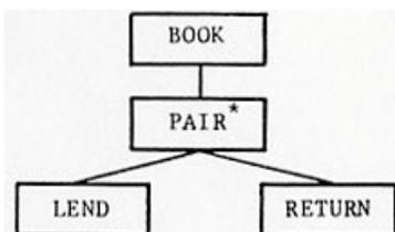
The asterisk in the box PAIR indicates that BOOK is an iteration of (consists of zero or more instances of) PAIR. In the second case, we wish to describe the behaviour of a customer of the same library. The actions are BORROW and RETURN, with obvious meaning; the constraint is that each BORROW must precede the corresponding RETURN, but BORROW and RETURN need not alternate. We must represent this constraint by two structures:
