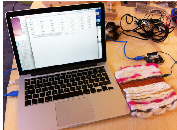
Figure 2: The technology set-up: a laptop running the SuperCollider application, an Arduino board with capacitive sensing and eTextile woven swatch connected by crocodile clip.
